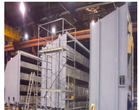
M&I's Air Intake/ Silencer Ducting for FR 7EA G.T.
